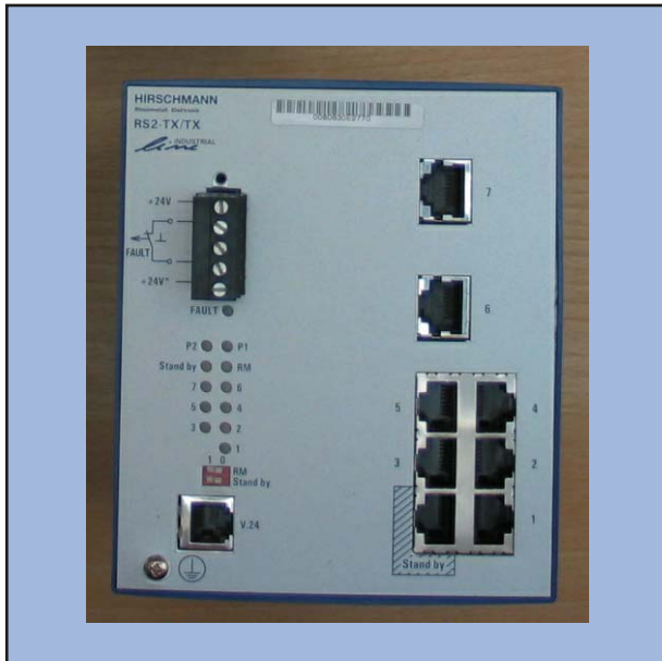
Picture 2: RAIL Switch
